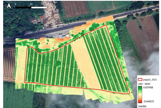
Fig. 5. Vegetation index NDVI applied on UAV images, pepper field (2021)
