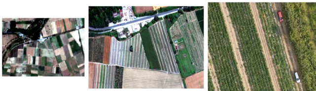
Fig. 3. Comparison of the different spatial resolution on the used data: From left to right Sentinel-2, 10m; WorldView-3, 0.31m; UAV, 0.03m
